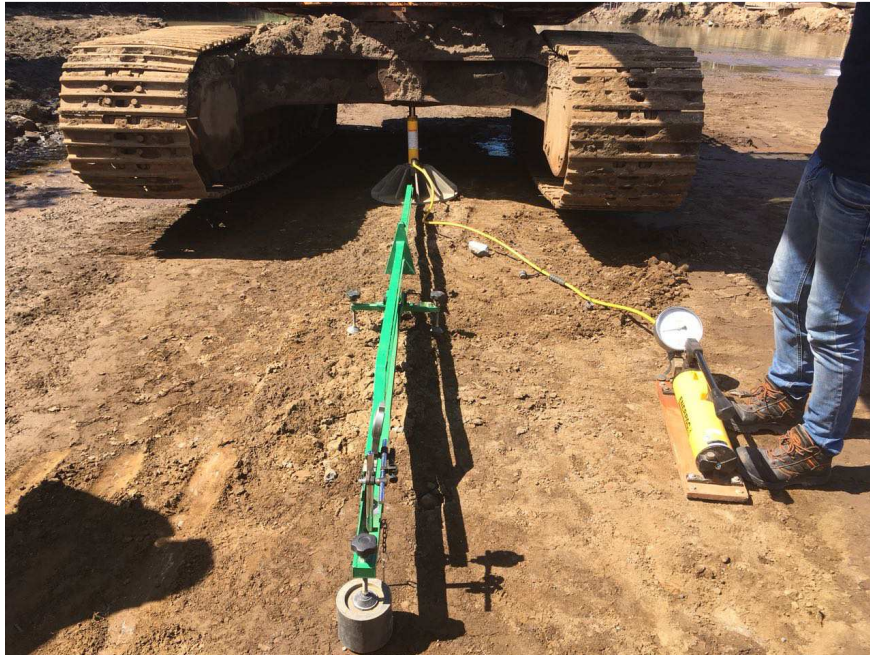
Figure 13: Plate Bearing test carried out on embankment
